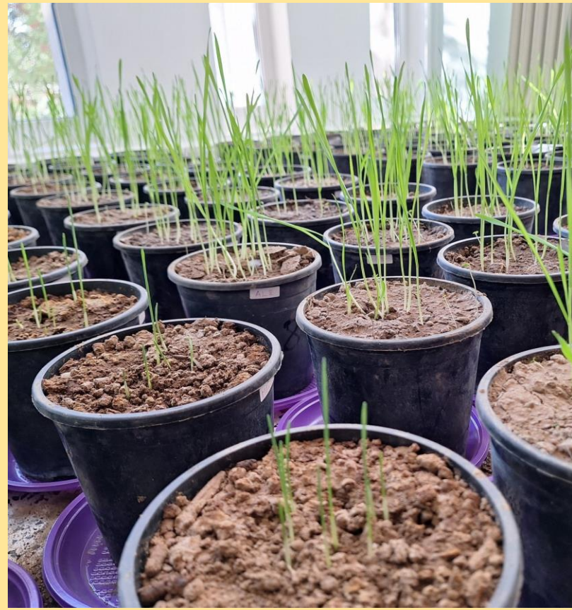
Creation and long-term water retention capacity testing of soil and mixtures in 120 pots
